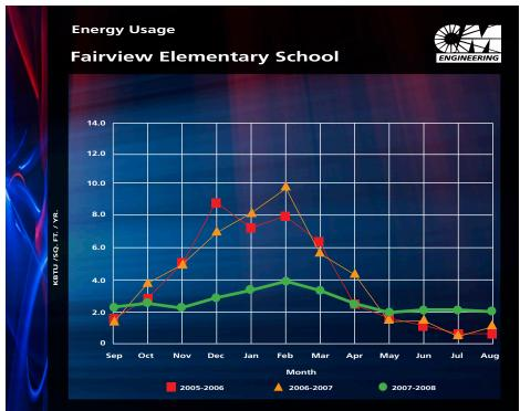
The green tracing above shows measured energy consumption after installation of One-Pipe Geothermal exchange heating and cooling system.
